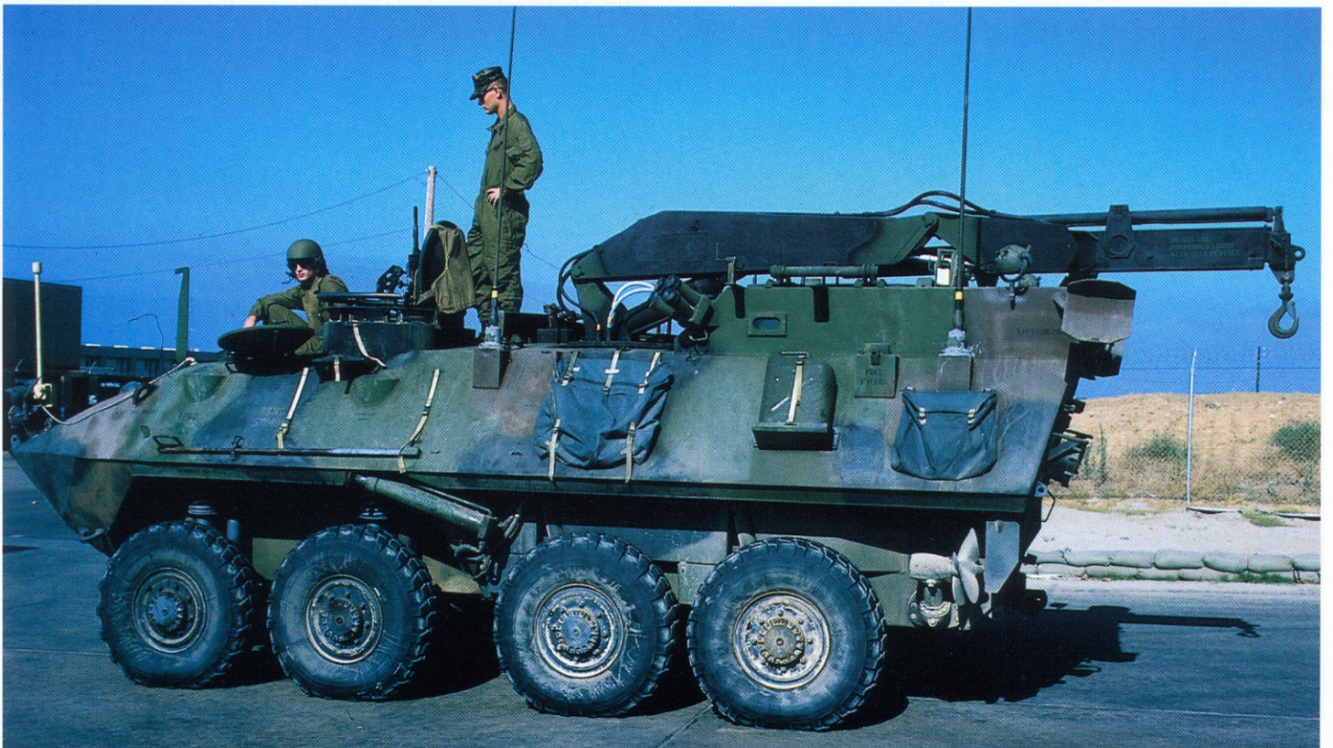
Bottom : View of the left side of the recovery LAV. The crane can lift 9,000 pounds and can traverse 265°.
